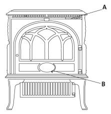
When first starting a fire: The primary control lever should be at the far right position, and the start-up air lever should be in the far right position. This will allow for the maximum amount of air to enter the stove and assist in starting the fire quickly and most effectively.
